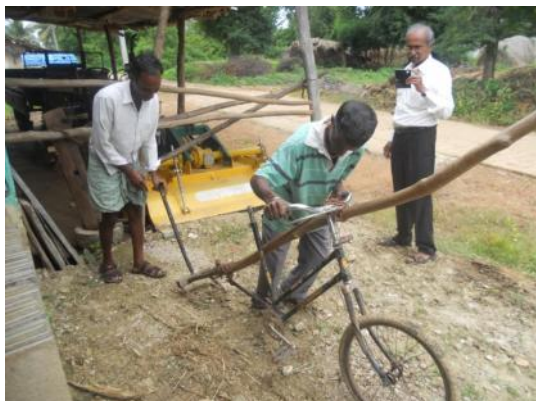
Local inter cultivator developed by farmers
